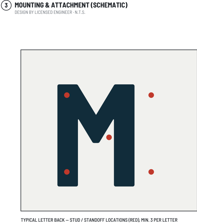
TYPICAL LETTER BACK – STUD / STANDOFF LOCATIONS (RED), MIN. 3 PER LETTER
