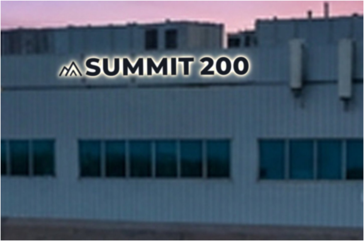
4 HALO ILLUMINATION (DUSK) 3000K WHITE - 200 max. NITS - STATIC - N.T.S.
